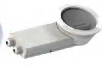
荧光灯 Fluorescent downlight 型号/Type:CWTD-5C(13W/18W/2x13W/2x18W) 尺寸/Size:φ177x393x77.5(mm) 防护等级/Protection class:IP44
